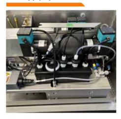
Our high flow recirculating ink supply system with exact temperature control and precise nozzle meniscus pressure control (ink flow rate) ensures optimal jetting operation.
