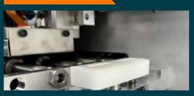
Versatex Printbars are fitted with a fully integrated maintenance station to ensure maximum uptime and lowest possible "make ready" time. As standard the Printbar has an auto maintenance module that applies suction to each printhead between job printing and with no manual intervention from the operator. The recirculating ink system can also be left in standby mode in any printing breaks, to enable agility and flexibility within
