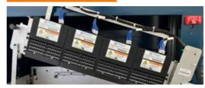
Integrated LED pinning offers users maximum flexibility for the final cure where required for the desired application. The power of pinning can also be fully controlled offering even more flexibility. A vacuum is included to extract any ink mist associated with printing, improving print quality by removing unwanted ink particles before they contaminate the substrate.
